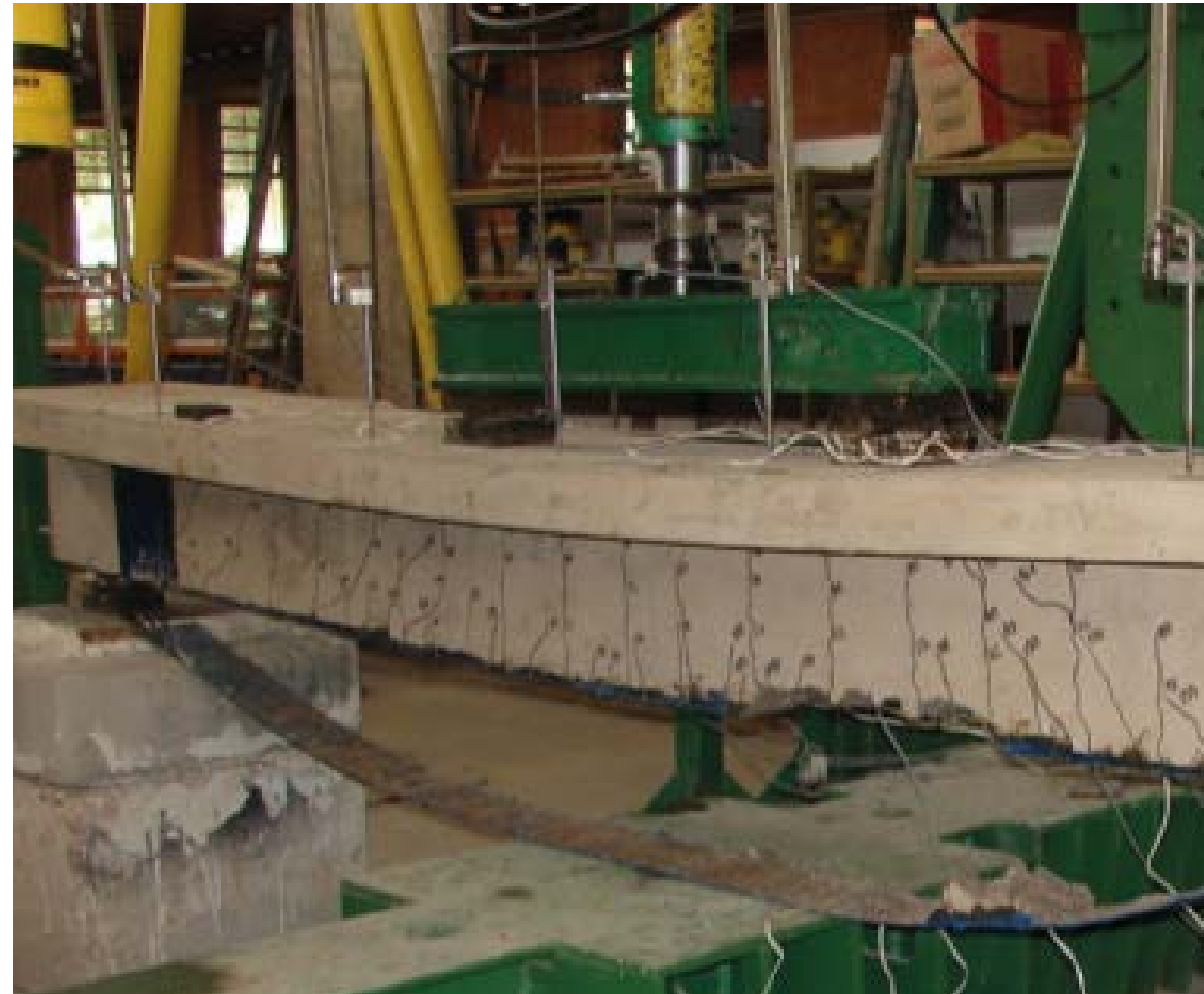
Figure 23. Peeling-off of Glass Fiber Reinforced Polymer (GFRP) laminate and rupture of concrete beam
